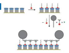
**Be specific:** A supramolecular adsorbate consisting of an adamantyl group (red) and an oligo(ethylene glycol) chain has been designed to prevent nonspecific protein adsorption at cyclodextrin molecular printboards. The adamantyl group allows specific and reversible interactions. Specific immobilization of proteins (gray) is possible through multivalent orthogonal linkers by effective replacement of the monovalent adsorbate (Ni<sup>2+</sup> ions (green) may be needed; see picture).
