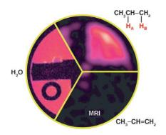
Gas-phase MRI phantom: Magnetic resonance imaging (MRI) in the gas phase was demonstrated using parahydrogen-induced polarization. H<sub>2</sub> enriched in the para (antiparallel) spin state and propylene gas were flowed over solid-supported Wilkinson's catalyst, and the product, propane gas, was collected in an NMR tube. Enhanced signal intensities were observed in the images of phantoms placed inside the NMR tube (see picture).
