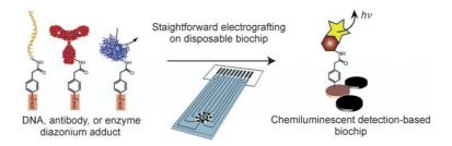
**Stuck on sensing**: A method is presented for the immobilization of aryl diazonium modified biomolecules by direct electrografting onto the surface of a conducting
